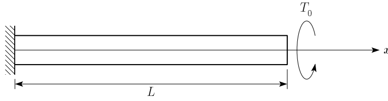
FIGURE 2.12 Cantilever beam with end torque
